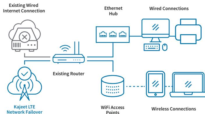
The solution can be easily integrated into your existing network infrastructure, and works with all the major North American wireless networks. Our backup Internet for businesses provides centralized data and device management and monitoring. Using policy controls, we ensure that neither data nor money is wasted on non-essential functions.
